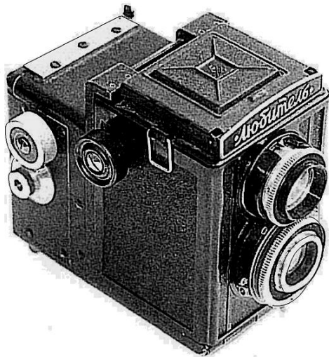
Elektron independently built-in electronic flash combining a Lubitel 2 camera and a Luch 57 flash, and Lubitel with high capacity 35mm film adapter
