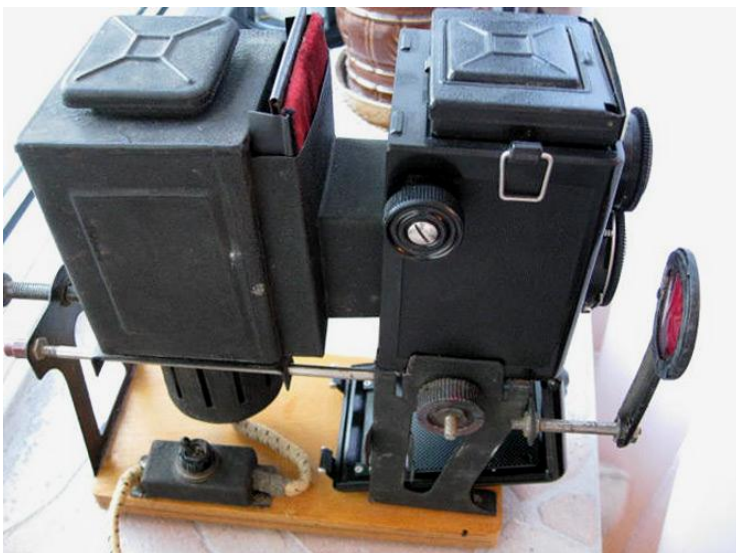
Device UPL-1 using the Lubitel body as enlarger part
