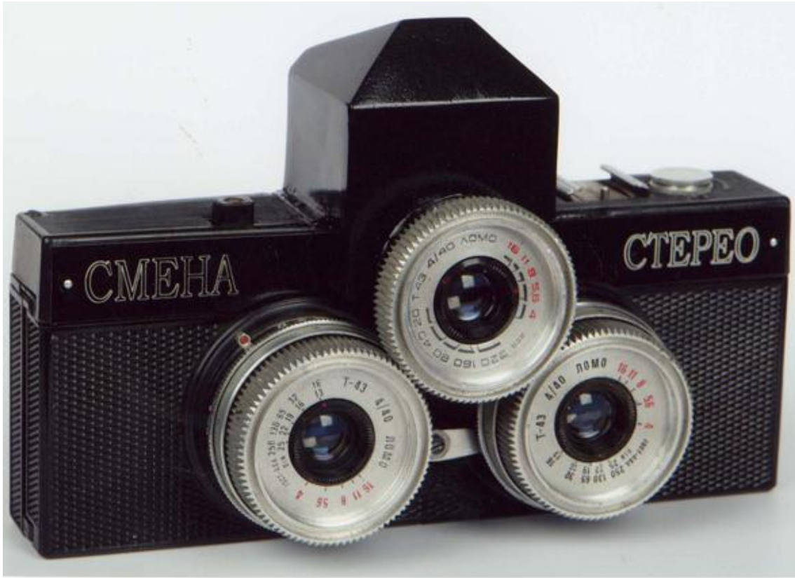
Smena Stereo factory prototype with reflex finder
