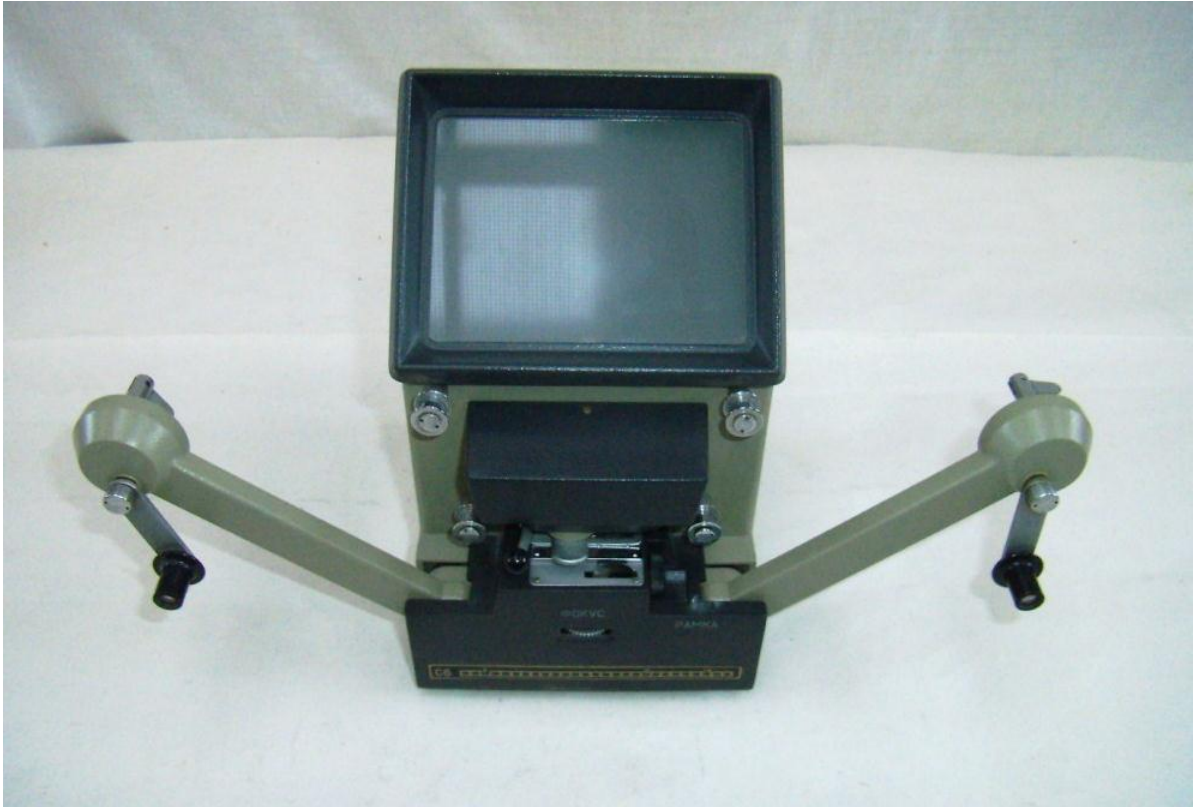
Kupava Amateur movie editor in three identical versions for 8mm, Super 8, and 16mm.
