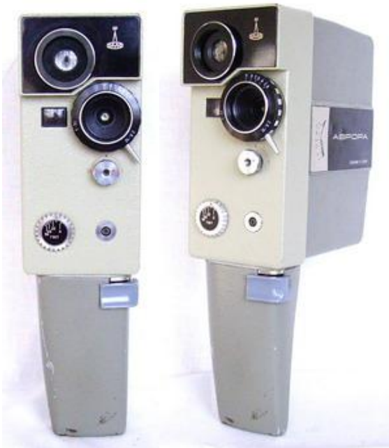
The Avrora grey or black was the electric eye version of the Sport 4 . -1966. T-51 2.8 10mm.
