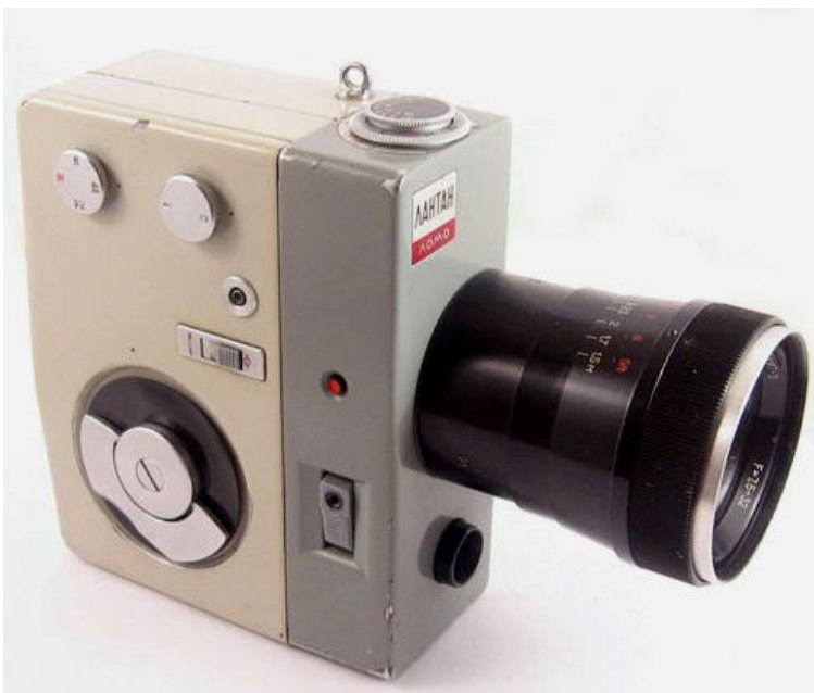
Lantan was the successor of the Lada Incorporates TTL auto electric eye. -1969. Granit-3 1.4 7.3/32mm
