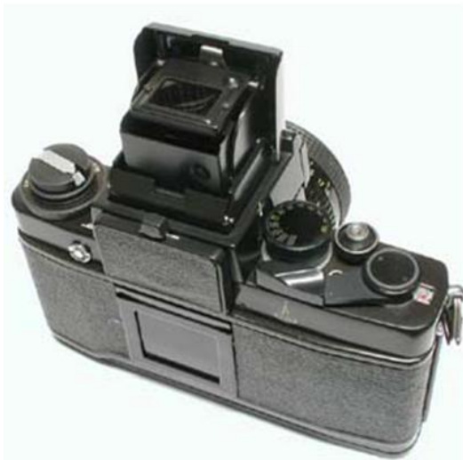
Right angle finder with diopter adjustment and folding finder
