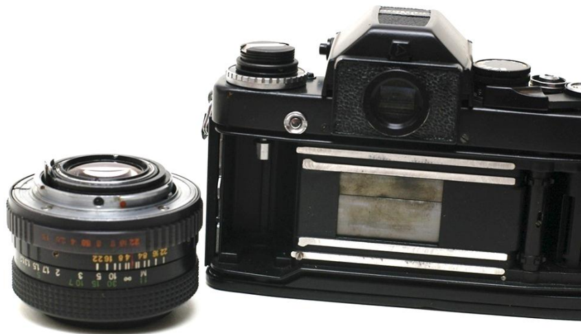
The four blade all metal shutter
