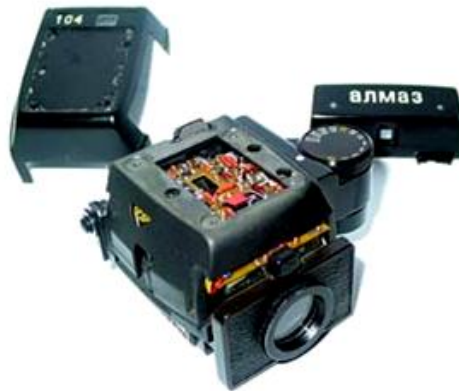
At left TTL prism of model 102 right from 104
